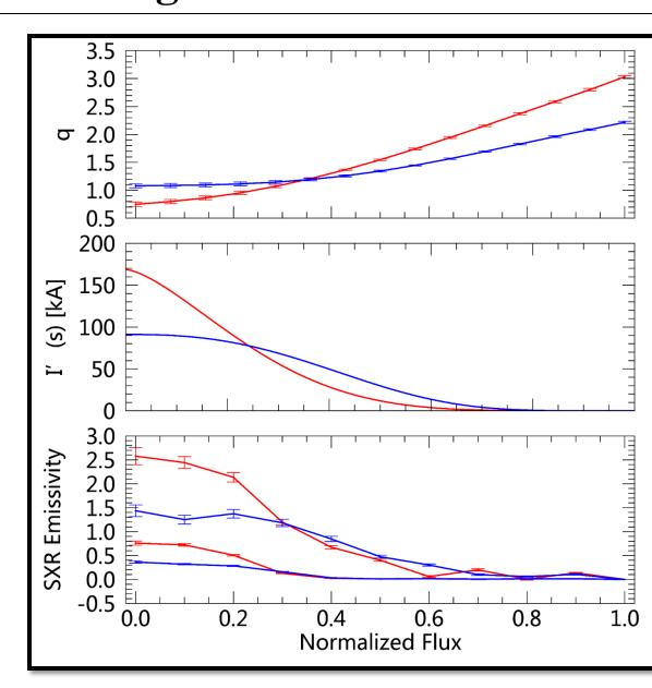
Addition of vacuum transform found to flatten both current and transform profiles, leading to a more stable regime.
