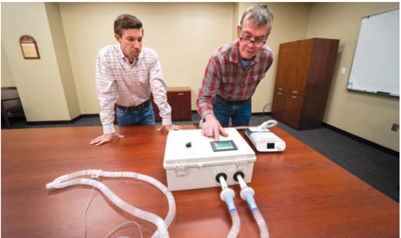
Michael Zabala, assistant professor in the Department of Mechanical Engineering, Samuel Ginn College of Engineering, and Tom Burch, lecturer in the Department of Mechanical Engineering, Samuel Ginn College of Engineering, examine the RE-INVENT accessory that would safely repurpose a CPAP into a functional ventilator. The design for this conversion was developed by a group of Auburn engineers as a quick and inexpensive way to convert CPAP machines into ventilators, one of the most important tools hospitals have for helping COVID-19 patients.
