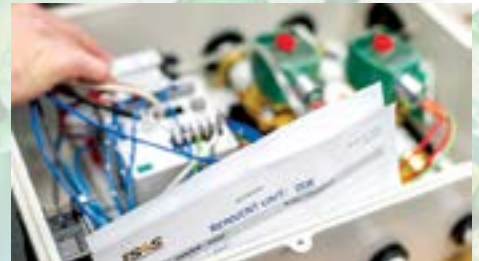
A partnership with Auburn University's Samuel Ginn College of Engineering, Integrated Solutions for Systems in Huntsville and the University of Alabama at Huntsville has led to production of the RE-InVENT, an innovative accessory that converts CPAP machines into emergency ventilators that was developed at Auburn to mitigate possible ventilator shortages across the country.
